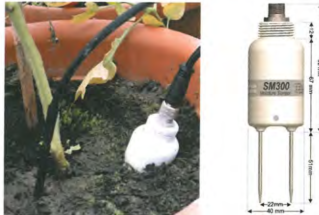
Fig. 2 – The experimental arrangement showing the close proximity of SM300 soil moisture sensor to the root zone of the tomato plant and the irrigation dripper.
