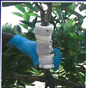
Sap flow meter-measures sap and water flowing throughout the trees. For research trials, the sap flow meter measures water uptake.
