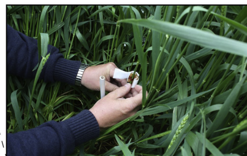
Fig. 1. (Top) External view of the minirhizotron facility located in Selhausen (Germany). (Middle) Internal view of the facility with the installation of rhizotron tubes at different depths. (Bottom) Example of the sap flow sensors used to estimate the transpiration fluxes.
