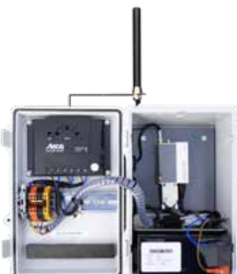
3G-DLC-BX1/SP modern gateway box (solar panel not shown)
