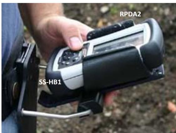
Rugged PDA with the Holster belt type SS-HB1
