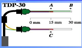
A- Thermocouple #1 B- Heater C-Reference Thermocouple
