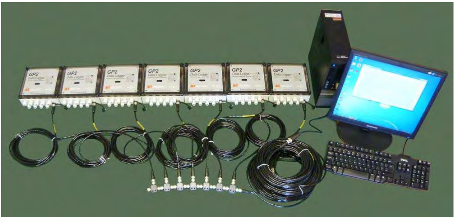
Figure A4. A network of 7 GP2 loggers connected to a PC via a total 100m of EXT/5w-xx extension cables and seven M12 5-way “GP2-NTP” T-Piece connectors. This is the maximum number of loggers and maximum cable length supported.
